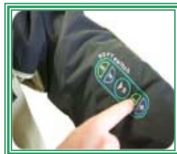
Figure 1: Integrated Textile Keypad (Softswitch, 2001)
